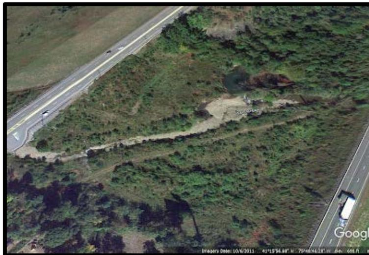
*Figure 19. Aerial View of the site in 2011 where Mill Creek diverted into the circular ponded area (north of the tan colored soils and rock in the center of the image) and infiltrated into the underground mine workings below.*
