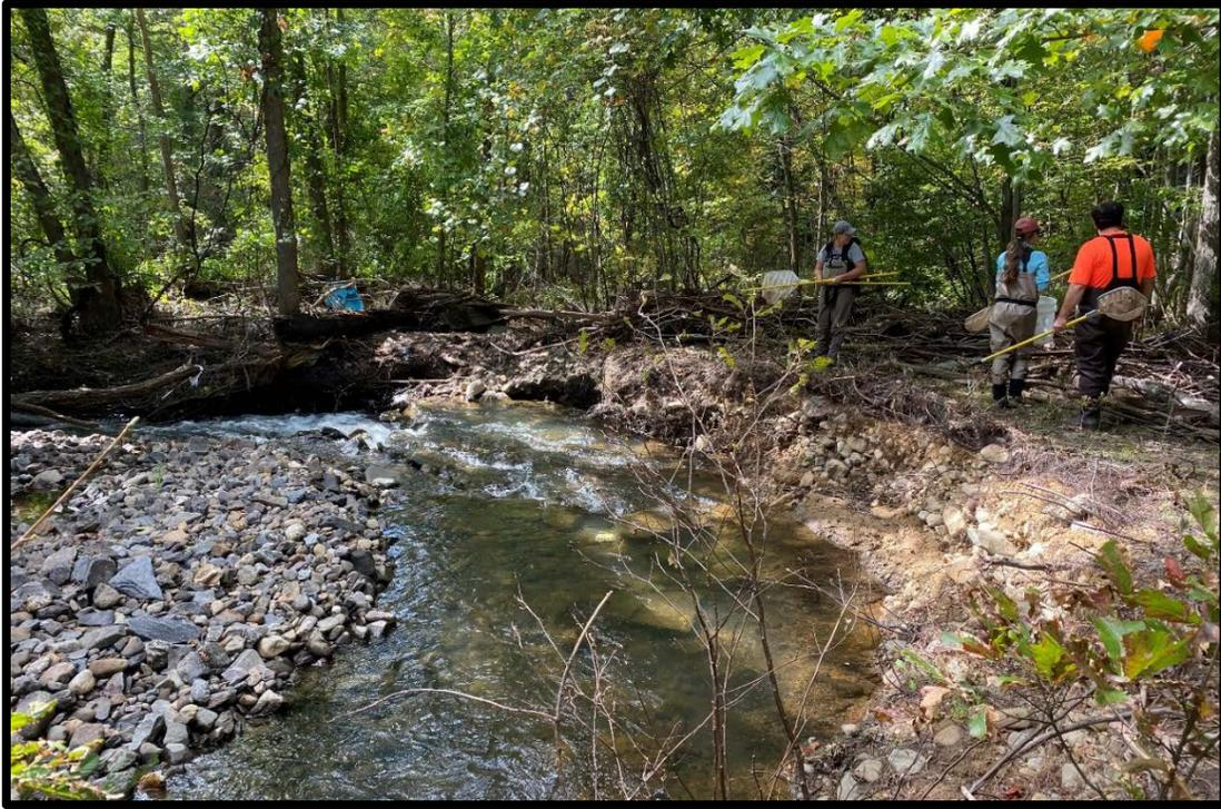
*Figure 85. A severely undercut streambank along Gardner Creek at Site 6*
